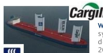
**Wing Sail system** - retrofit + operation system = 30% fuel saving - detailed design stage - installation on 1st tanker 2022 - EU CHEK H2020 project launched Q2 2021
