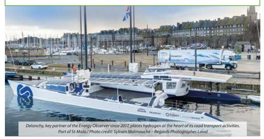
Here you see the Chereau Hydrogen Power H2 semi used by DELANCHY in real conditions of use; a trailer whose cooling unit is hydrogen powered.
