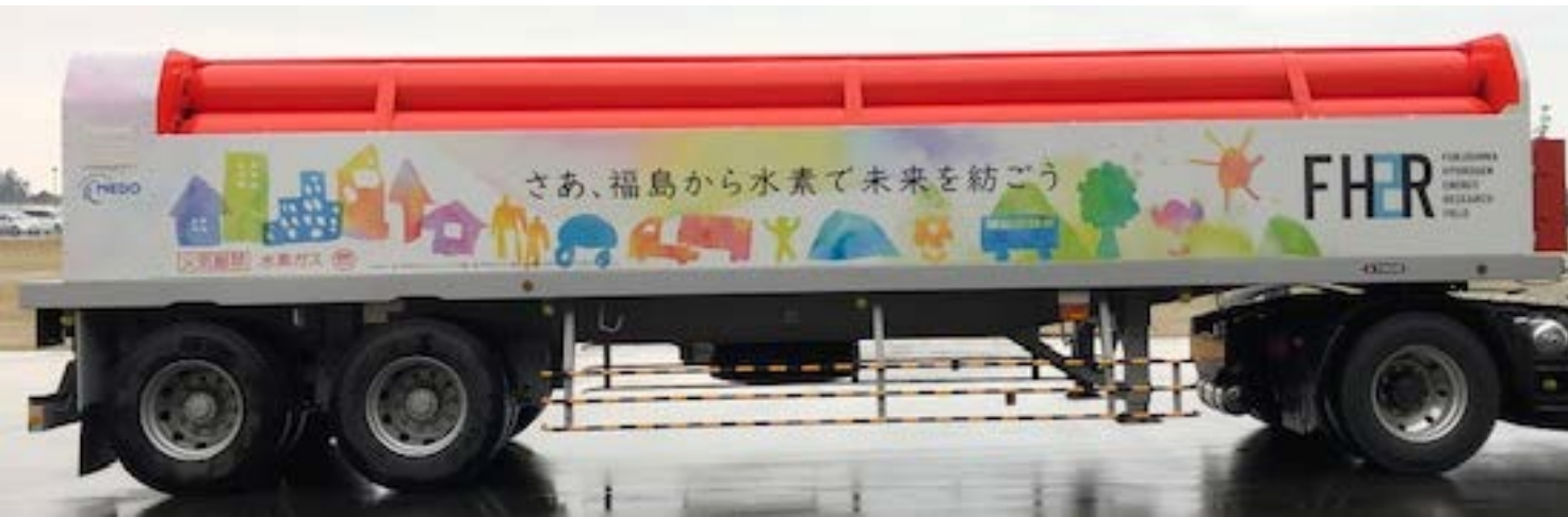
Tube Trailer (capacity : 0.237t(2,642 Nm3))
