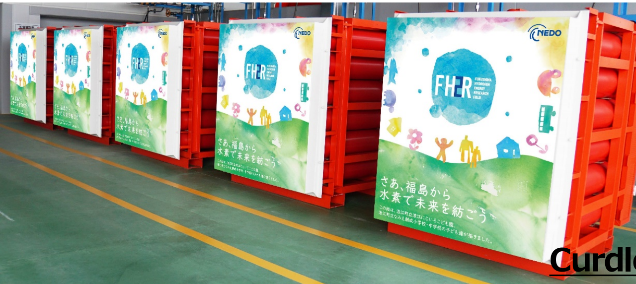
Tube Trailer (capacity : 0.237t(2,642 Nm3))
