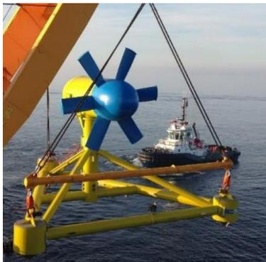
**Figure 6.** Hydrolienne Sabella D-10 In-stream.
